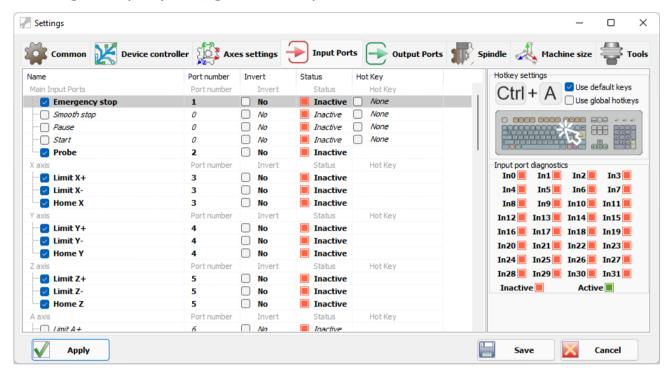
Set the input port numbers according to the configuration of the machine and the CNC controller.
