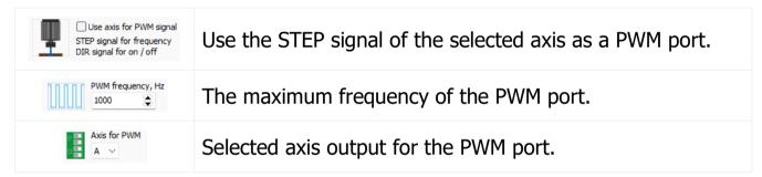
To change the PWM frequency, use M-code M3 or M4 with S, M3S1000. The "PWM frequency" setting has a linear relationship with the "Spindle speed" setting.
