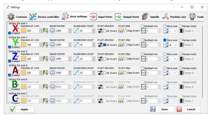
Set the required number of pulses for each axis. If necessary, specify the subordination of the axes and change the direction of movement.
