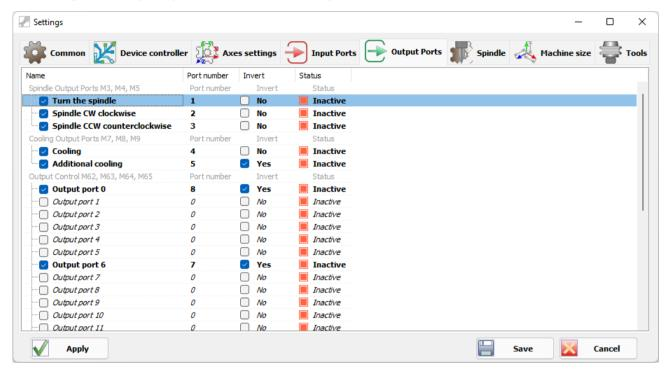
Set the output port numbers according to the configuration of the machine and the CNC controller.
