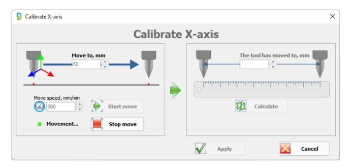
After the tool has finished moving, use the ruler to measure the actual distance the tool moved. Enter this value in the "The tool has moved" to field.
