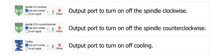
With this **Counterclockwise/Clockwise** setting, you can set the direction of rotation of the spindle when you press the "Turn the spindle" button in the main window.
