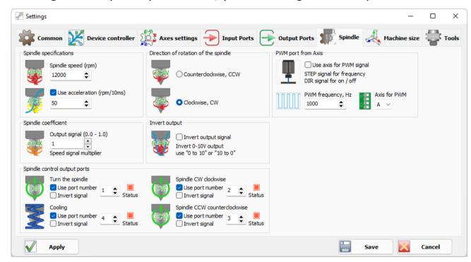
Set the speed and acceleration parameters according to the spindle specification. Set the default spindle rotation direction.
