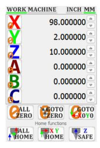
To reset the axis coordinate to zero, click on the corresponding button depending on the selected axis.
