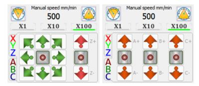
This field sets the speed of movement of the instrument during manual operation. C
