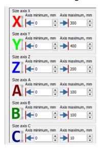
According to these settings in the 3D model window, the dimensions of the axis will be displayed as a quadrilateral in each plane.
