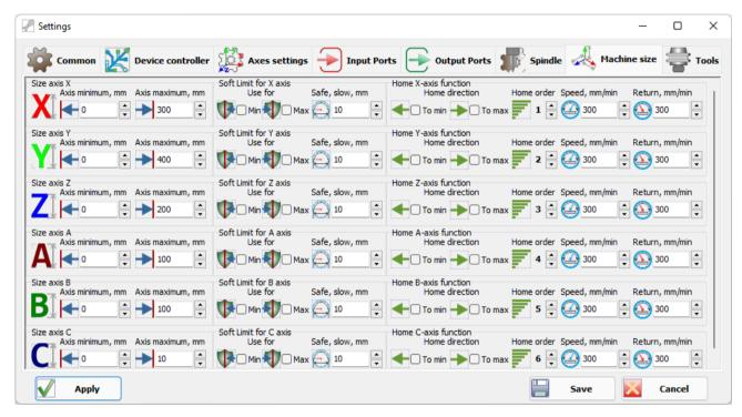
These settings are used to display machine limits in the 3D model window. For the operation of safe limits and the operation of the HOME function.
