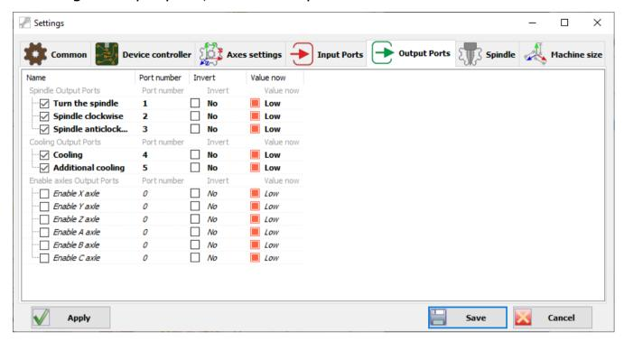
Set the output port numbers according to the configuration of the machine and the CNC controller. Save the settings.
