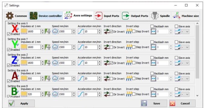
Set the required number of pulses for each axis. Save the settings. If necessary, specify the submission of the axes. Use the inversion setting to change the direction of rotation of the motor.
