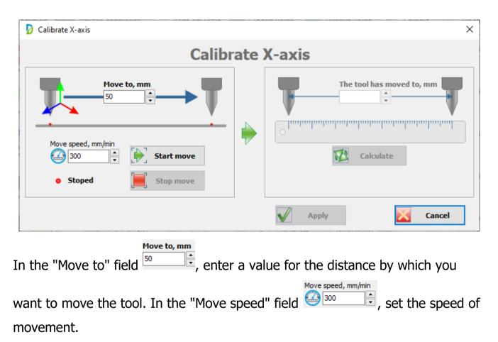
Attention! This speed must be slow! This is necessary so that you can quickly respond to an emergency and not damage the machine.
