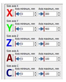
According to these settings in the 3D model window, the dimensions of the axis will be displayed as a quadrilateral in each plane.
