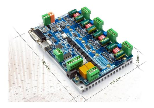
The bottom install size is 142.6mm\*96mm.
