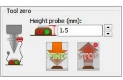
For the tool zero search to work correctly, you must set the input port number in accordance with the port number on the controller where your probe is connected. Set "Invert" so that the "Value now" in the normal state of the Probe is "Low".
