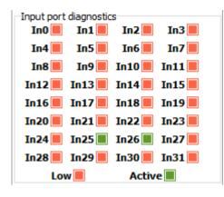
A red LED indicates I there is no signal on the input port. A green LED indicates I signal is present on the input port.
