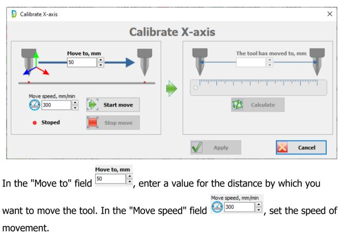
Attention! This speed must be slow! This is necessary so that you can quickly respond to an emergency and not damage the machine.
