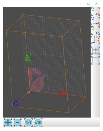
To rotate the 3D model, move the mouse pointer to the display area of the 3D model. Right-click and hold to move the mouse pointer. You can also use
