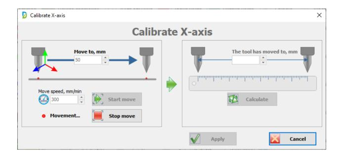
After the tool has finished moving, use the ruler to measure the actual distance the tool moved.
