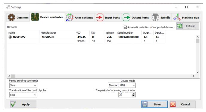
In the hardware section, you must select a controller by setting a point in the radio button block opposite the USB controller. Save the settings.
