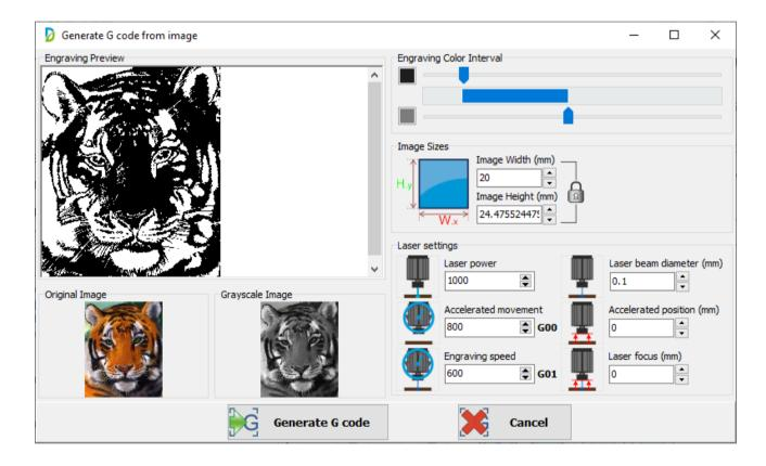
In the engraving color interval block, you can adjust the color interval.
