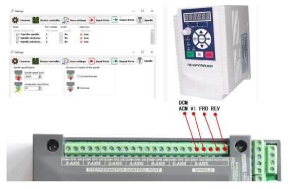
**3 -** Common IO output include OUT1, OUT2 on the spindle interface, totally 10 ports IO output, open drain output.
