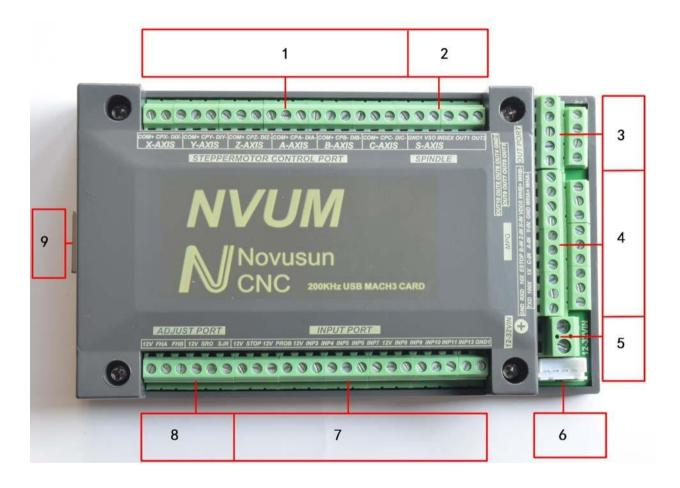
**1 -** Terminal block is 6 axis stepper driver control output interface, from left to right, there are X,Y,Z,A,B,C 6 axis output, it's common anode, the cable connection for each axis is COM+/CP-/DIR-, COM is common+ ,CP is Pulse-, DIR is direction-.
