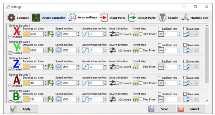
Set the required number of pulses for each axis. Save the settings. If necessary, specify the submission of the axes. Use the inversion setting to change the direction of rotation of the motor.
