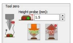
For the tool zero search to work correctly, you must set the input port number in accordance with the port number on the controller where your probe is connected. Set "Invert" so that the "Value now" in the normal state of the Probe is "Low".
