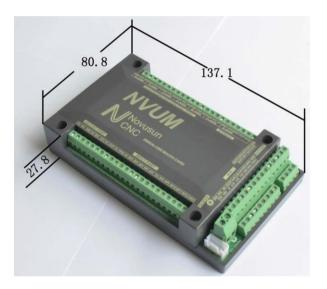
The bottom install size is 101.4mm\*39.5mm
